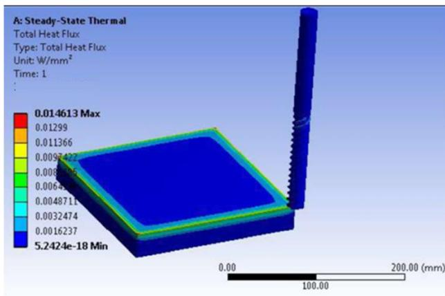
FIG: Heat flux at 460k
